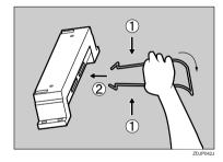
Insert the claws of the stand into the holes on the left side of the printer (①), and push down (②).
