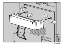
Open the front cover slowly by pulling the two points on the left and right.
