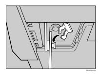
Make sure the auxiliary bar and stopper are installed in the positions shown in the illustration.
