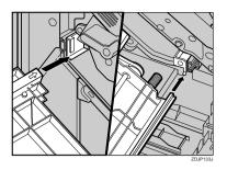
Fasten the Duplex Feed Unit with one short screw using provided screwdriver.
