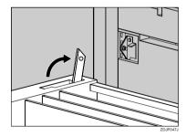
Hook the hole of the auxiliary bar on the mounting bracket of the printer.
