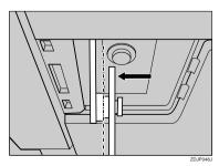
In step 5, move the auxiliary bar to the position shown with a perforated line in the illustration.
