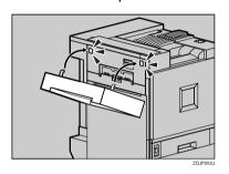
Remove the adhesive tape which hold the cable, and then connect the cable of the Duplex Reversal Unit to the upper connector on the back of the printer.
