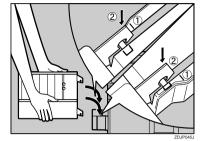
The hooks of the Duplex Reversal Unit grasp the bar inside the groove of the stand.
